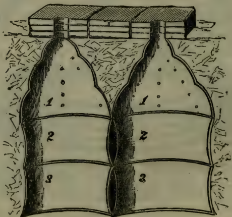
Section of drain.
